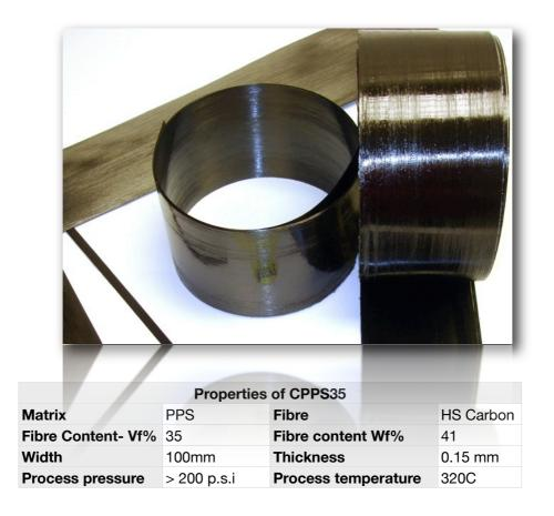
AtenPly, is a continuous, fibre reinforced thermoplastic composite prepreg tape, made direct from the fibre roving and thermoplastic melt to produce a light weight, high-strength, well impregnated tape with unidirectional fibre reinforcement. AtenPly is made to standard widths and thicknesses but other sizes, fibre volume fractions etc are available on request.
